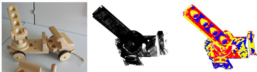
(a) Wooden toy firetruck. (b) Point cloud of scanned firetruck. (c) Point cloud of firetruck colored by primitive class.
