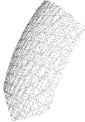
Fig. 2: Point cloud patch of a sphere.
